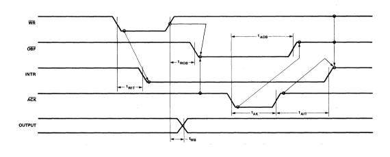
Figure 29. MODE 1 (Strobed Output)
